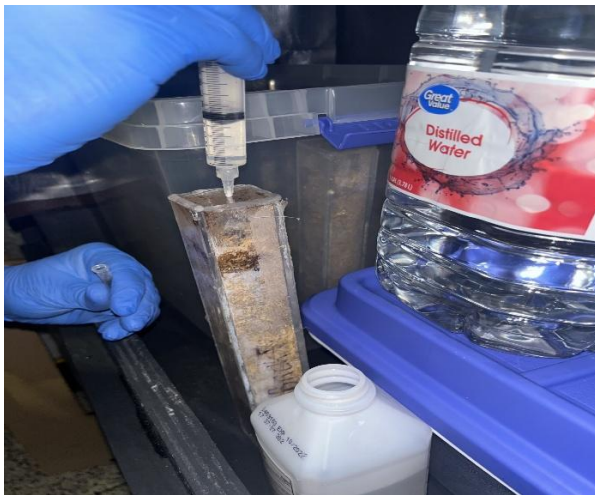
Sterile watering of bricks with a syringe (30 mm)
