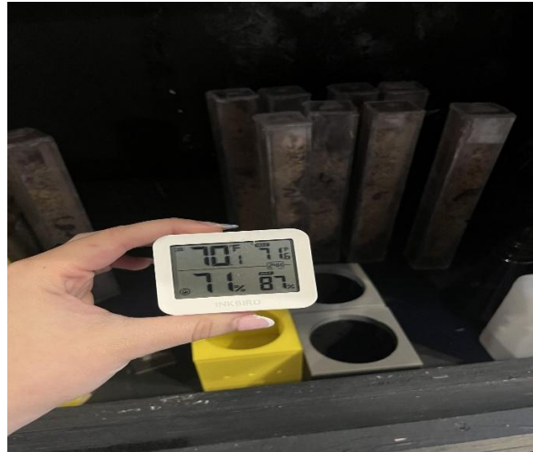
Humidity and temperature tracking
