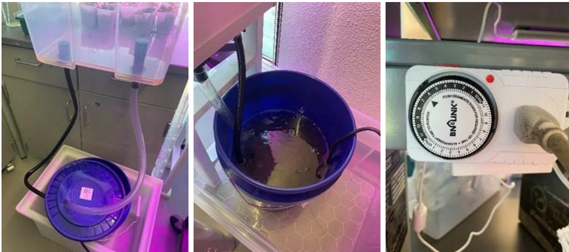
Figure 1. Irrigation system (Watering cycle: 7:30 AM and 8:30 PM)
