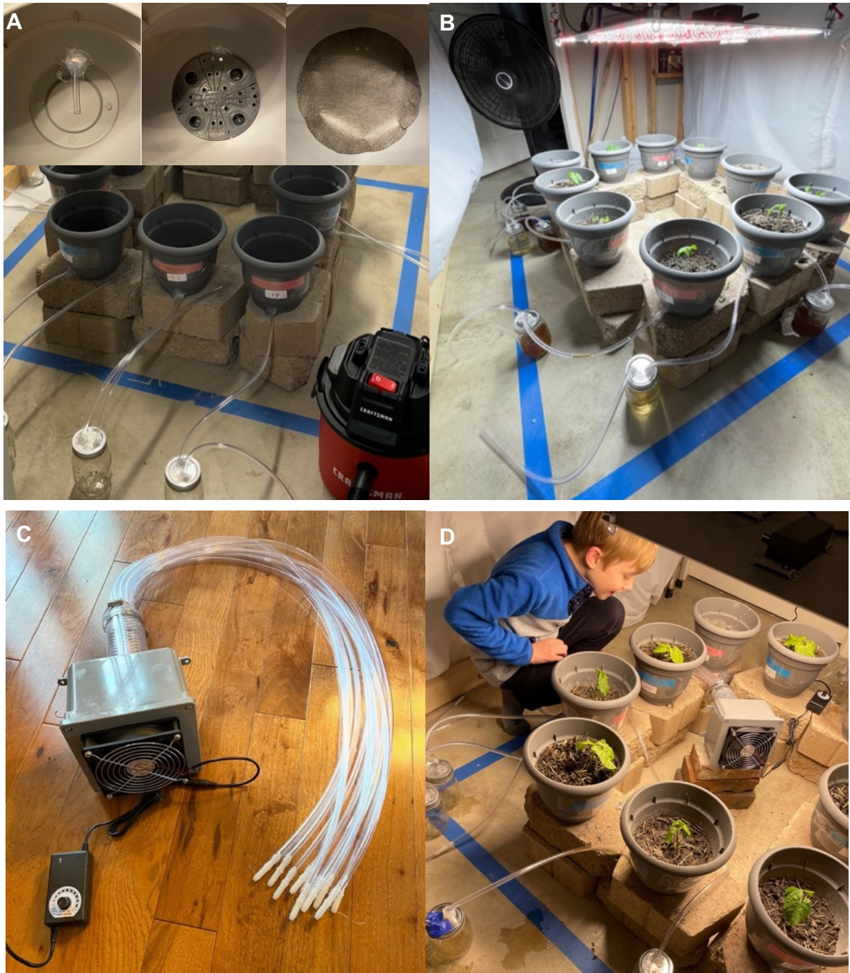
FIGURE 4. Novel Soil Atmosphere Circulation System. (A) Low Gravity Drainage Enhancement System (LGDES), (B) 18-inch diameter pedestal fan, (C) Subsurface Atmosphere Ventilation System (SAVS) before installation, and (D) SAVS after installation.
