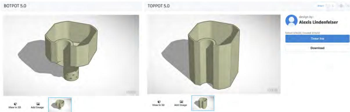
**Figure 5:** The final 3D-models (in Tinkercad) of both pieces of our pots. They would be later glued together and placed on top of the reservoir. The semicircle cutout in the side enables water to be poured into the reservoir to refill it without lifting up the funnel and disturbing the plants.
