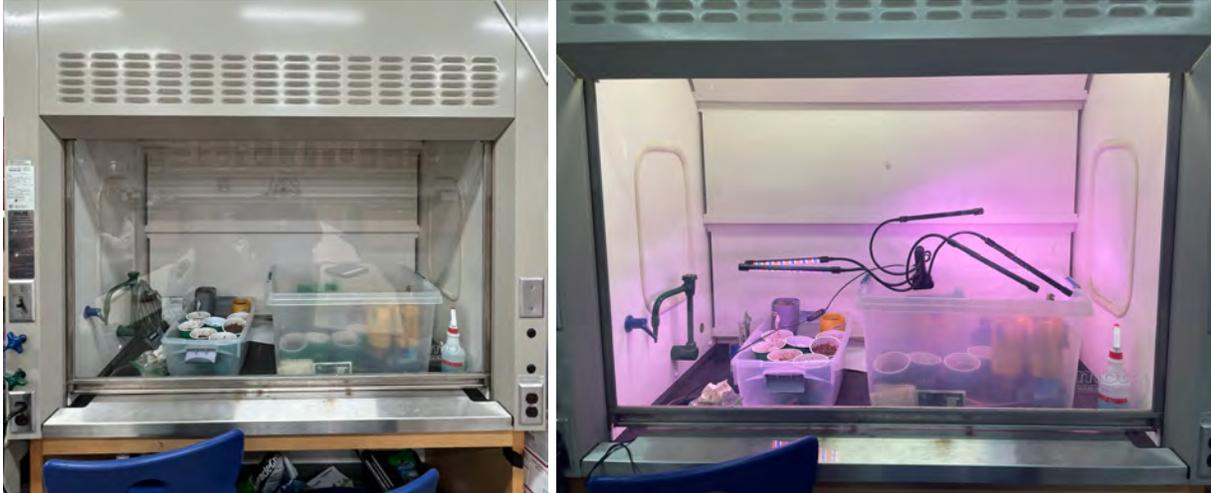
**Figure 4:** The outside of the fume hood and the setup, with red and blue LED grow lights.
