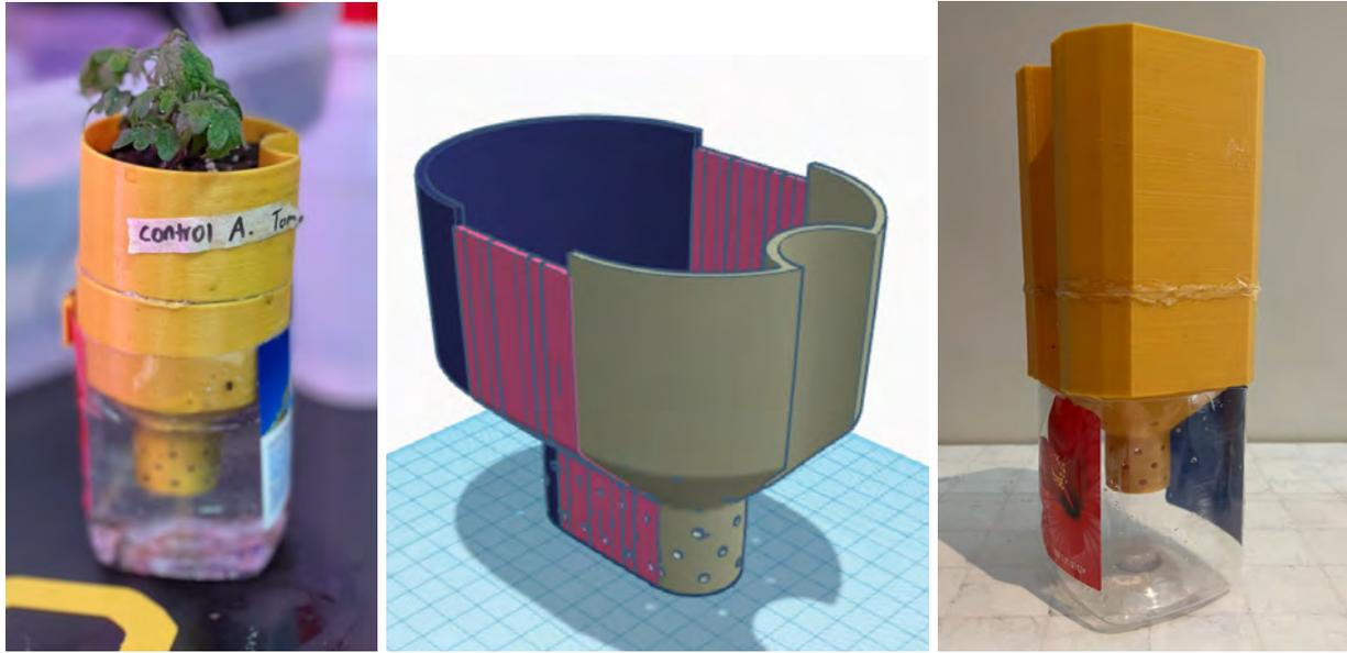
**Figure 6:** Multiple iterations of our pots. **Left:** The second iteration was redesigned because it was too small. **Middle:** The third iteration, oblong to maximize volume, but impractical for a reservoir. **Right:** The final iteration, finding a perfect balance between size and shape.
