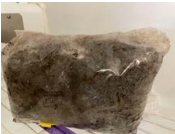
Image 6b: Bag 5 75% OM/25% MSG-1 Substrate Mixture Midway Image (33 days)
