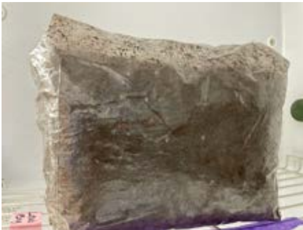
Image 6b: Bag 5 75% OM/25% MSG-1 Substrate Mixture Midway Image (33 days)
