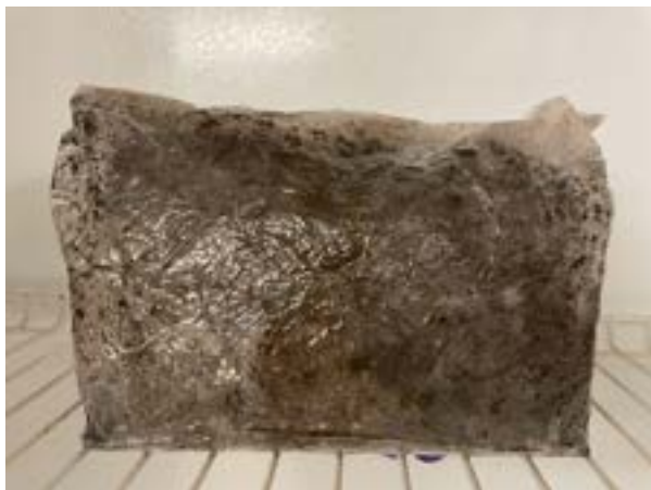
Image 5b: Bag 4 80% OM/20% MSG-1 Substrate Mixture Midway Image (33 days)
