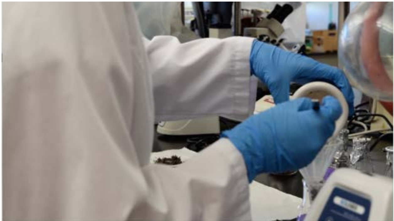
Figure 8: A member of the team transferring ground up samples for pH data collection.
